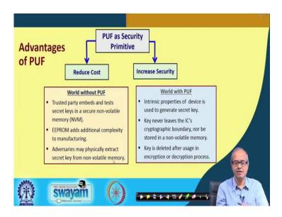
So, talking about the advantages of PUF, if you talk about PUF as a basic building block, you are using to design secure hardware, there are broadly two things – it reduces the
