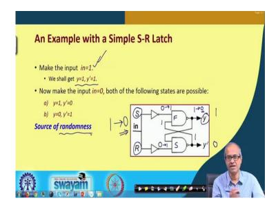
Let us take a simple example of an S-R latch. I will just try to explain what this fabrication dependent or device dependent variations mean. Well, if you recall for those of you know how an S-R flip flop works; this is a single bit storage which store 1 bit of information, ok. There is one input "in" that same input is fed to this S and R let us say. This S and R are two different inputs; let us assume that the same input value "in" is fed to both S and R.
