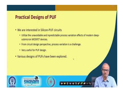
Now, in terms of the practical design, how the PUFs are actually implemented? Well, we are interested in chips right. So, we are interested in silicon PUF circuits which are implemented in silicon or CMOS. As I had said the basic idea is that when you fabricate chips, there will be process variations; from one chip to the other there will be some variations. So, those variations are exploited here.
