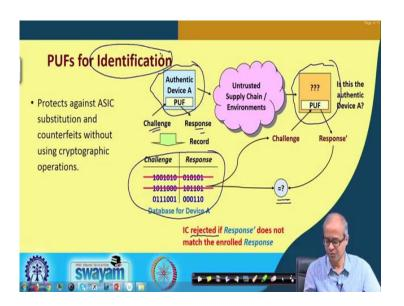
There is another application of PUF where you want to identify; like I have fabricated or I have designed the device and someone has made a clone or a copy of my device; I want to find out which is the original and which is the copy. You see, for the authentic device which I had designed, I know what was my challenge/response properties. Let us say I have already created a table like that; this is the, for this challenge, this will be the response; for this challenge this will be the response.
