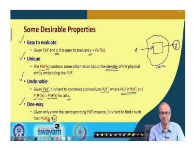
Some of the desirable properties of PUF are mentioned here. These are quite obvious. First is it should be something which should not be too difficult to evaluate in terms of the challenges response. Suppose, I give a challenge x, the response y should be easy to calculate, easy to compute ok. It should be easy to evaluate.
