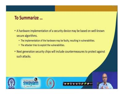
So, to summarize the hardware implementation of some algorithm that goes inside the security device, this is of course, based on some well known algorithm; typically some cryptographic algorithm. The point is these algorithms are known to be very good, but the way they are implemented in hardware that may not be very proper; that may have some vulnerabilities or weaknesses.
