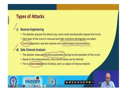
Now, the third kind of an attack which is very sophisticated, this is called reverse engineering. Now, for those of you who have some idea regarding how an IC chip is fabricated; you may be knowing that you start with the silicon base that is called an wafer and on a silicon wafer layer by layer we put lot of depositions. There are various layers which are put like diffusion, polysilicon, metals, contacts. So, it is like a building that is being constructed on top of that silicon wafer.
