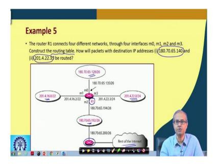
Let us take one last example. So, here we consider a router R1, this is our router R1. So, as you can see, there are four interfaces m0, m1, m2 and m3 and these are the networks which it is connected to, these are the network addresses and also in CIDR notation, number of bits of the network address is also mentioned 26, 22, 26 and here 24.
