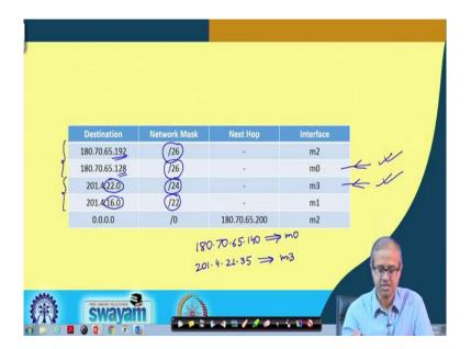
So, I am actually showing you the solution, you can just verify, for the first network through m2 which is connected to m2. If you recall there are 26 bits of the address. So, it is slash 26 and this is the network address, through m0 also there is 26 bits like this m3, m1 and finally, m2 is the default which we will be sending it to the external router.
