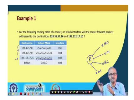
The first example that we take here, is something like this. Let us assume that we have a router, let us say we have a router which has four interfaces. There are four links to the router and this interface names we are giving as eth0, eth1, eth2, eth3. Now this eth is the short form for Ethernet, because typically inside a LAN this interfaces are typically Ethernet networks, so that is why we are giving this names like this eth0 to 3.
