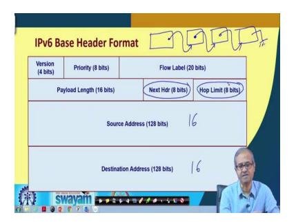
Now, the base header, 40 bytes, will be having a fixed structure like this, which is some of the fields or somewhat similar to, I mean IP version 4, but because of the change, size of the address as you see, source address and destination address are 128 bits long. Well 128 bits means how many bytes? 16 bytes, you have 16 bytes here, you have 16 bytes here, version is 4 bits.
