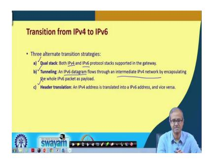
So, talking about transition to IPv4 to IPv6, due to the incompatibilities, there are challenges, but there are broadly three approaches you can think of; one is you implement both IPv4 and IPv6 protocols in the router or the gateway, so that if someone wants to use or send IPv4 packets it can be handled, v6 packets can also be handled something like that.
