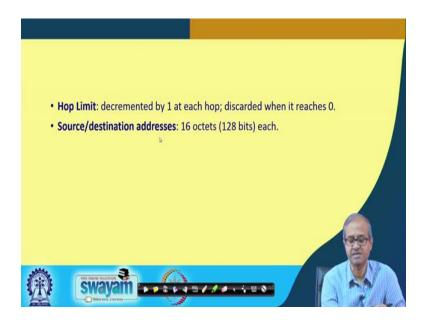
Hop limit; similar to IP version 4, it is decremented by 1 at each hop and the addresses are 128 bits or 16 bytes or octets ok.
