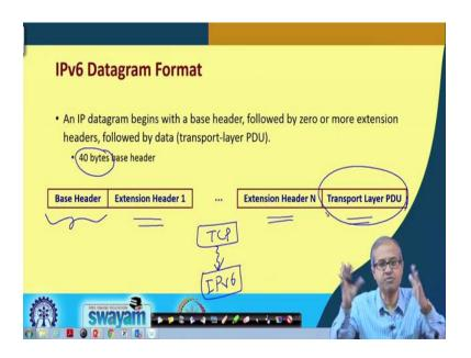
So, IP datagram format as I had said, there can be multiple extension headers, the general picture is like this, it starts with the base header which is 40 bytes in size, but there can be multiple extension headers, the size of the extension headers can be different and at the end, you have the data, because typically let us say TCP is running on top and below you have this IP version 4/6 running, IPv6.
