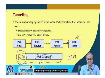
So, this is what tunnelling is all about, which was used in the previous case. So, here diagrammatically it is explained. So, you have an IP version 6 host which is generating an IP version 6 packet. Then you have to send it to IPv4 router, what to do? You append an IPv4 header before it.
