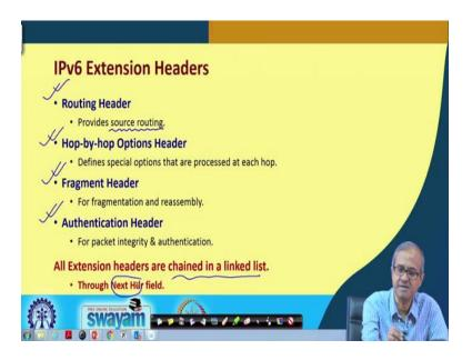
Now, the important kinds of extension headers which are there, they are summarized here, there can be a routing header as your seeing here. Routing here, routing header permits source routing. No I am repeating here, what source routing actually means. Now in the conventional packet routing what happens?
