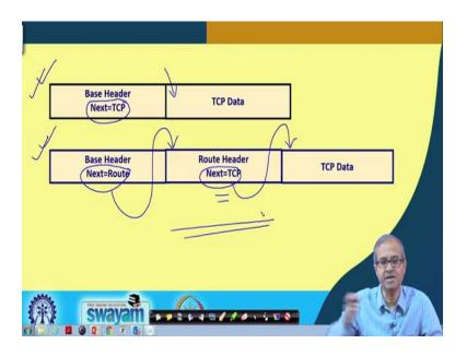
So, pictorially it will look something like this. This is one example, suppose this is a IPv6 packet which does not contain any extension header. So, in the base header, the relevant fields are there and the next header field contains TCP, which means it will know that the, that whatever follows the base header is the actual TCP PDU which is carrying the data to be transmitted.
