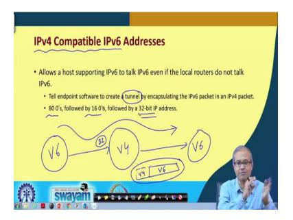
Similarly, you can have another option which is called IP version 4 compatible IP version 6 address. Here it is something like this, suppose there is a network running version 6, there is another network running version 6, but in between there maybe routers through which the packets are flowing, they may be version 4 compatible. So, how will this version 6 packets flow in this network?
