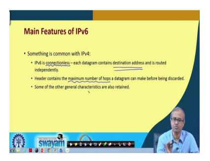
So, main features of IPv6, few of the features are borrowed from IPv4, whatever was there, same thing is carried forward. First such thing is connectionless, IP version 4 was based on datagrams, IP version 6 is also based on datagrams, which is a connectionless protocol.
