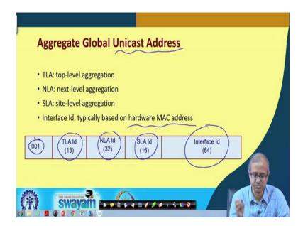
Now, talking about the 128 bit address, you see this 128 bit address is typically separated using a number of hierarchies. The last 64 bits here, this specifies something similar to the host address path in IP version 4, it talks about some kind of unique addressing inside the network that you are addressing.
