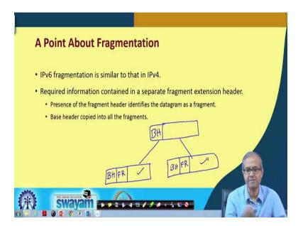
Now, about fragmentation just as I mentioned, this IP version 6 fragmentation is similar to IP version 4, but unlike IP version 4 where the additional information or fragmentation was put inside the same header, here we are using a separate extension header. So, when a fragment get, there is at when IP version 6 packet, let us say there was a packet which had a base header, let us say BH, when it gets fragmented into two pieces, the scenario will be something like this.
