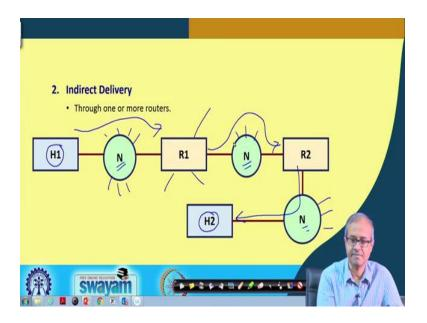
Then comes indirect delivery. Indirect delivery means the source and destination are not part of the same network. They belong to two different networks. So, as this diagram shows, let us suppose this H1 wants to send a packet to host H2. So, as you can see, there are three networks. Here, this N means networks. There are three networks, but I have shown only some, there can be other connections also to the network, other hosts and routers. There can be connections ok. So, I have shown only few.
