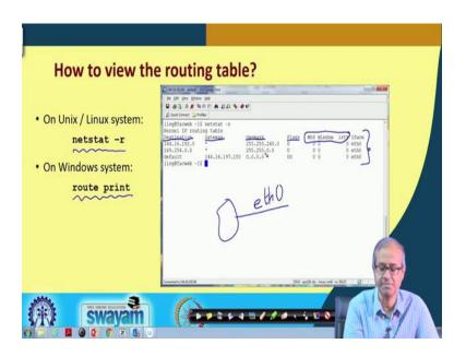
Now, the question is in a computer or in a router how do we view the routing table. Let us say on a computer if you are, if you are using a Unix or a Linux system, then the most command to use is "netstat – r". Similarly on an windows system there is a command called "route print". It will print the routing table of that computer. Like in this screen, well the entries are very small, you may not be able to read clearly.
