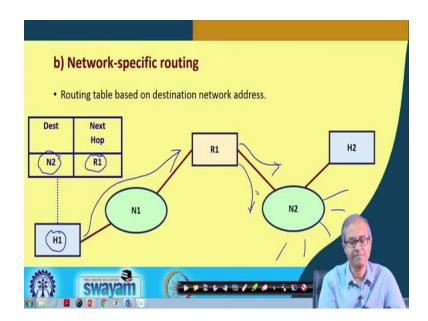
Then network specific routing, I said sometimes I specify the address of a network as a destination rather than a, sorry rather than a host. So, I can specify the address of a network as the destination. So, suppose from host H1, I am sending a packet, I am specifying I have to go to N2. It can be a broadcast packet, it will be broadcast to all the hosts in N2.
