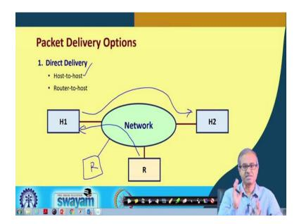
Now talking about the packet delivery options, I am particularly talking about the IP layer here, because as I said, TCP/IP is the most dominant protocol that drives the Internet and IP is the most widely used protocol at the network layer level which is responsible for packet routing. So, when you talk about packet delivery options, we are talking about a scenario like this as I have shown in this diagram.
