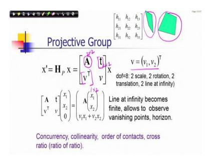
So, the parent group which is a projective group that is represented in this form. You can see that it is a  $3\times3$  matrix, but we are representing it by their sub matrices where A is a sub matrix of  $2\times2$  sub matrix. So, this is a  $2\times2$  sub matrix. And t is  $2\times1$  column vector, V transpose we have already shown how V should be represented its a column vector of  $(v_1, v_2)^T$
