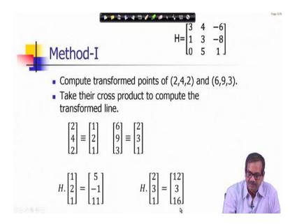
So, first let me reduce the representation of this points. Since, there is a scalar quantity 2, I can divide all the coordinates to make it more simple representations of (1, 2, 1) and similarly (6, 9, 3) I can simpler representation of (2, 3, 1), you could have performed using (2, 4, 2) and (6, 9, 3) also. So, it is just for the convenience of the computations I have taken these two. Now, you transform (1, 2, 1) and (2, 3, 1). So, if I transform
