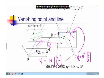
So, let us discuss again that how vanishing points they are related in the transformation, in the transformed space. So, in this case we have drawn a pair of parallel lines and one of them is denoted by l. Consider l is transformed in the transformed space by a line l' and we know how l and l' is related. So, you multiply l, represent it in a two-
