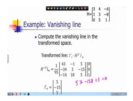
So, here as we discussed that vanishing line could be computed by transforming the line at infinity of the original projective space which is incidentally  $\begin{bmatrix} 0 \\ 0 \\ 1 \end{bmatrix}$ . So, we will be computing, we will be performing this computation and if I multiply the corresponding transpose of this inverse with  $\begin{bmatrix} 0 \\ 0 \\ 1 \end{bmatrix}$ , then you will get the corresponding vanishing line as
