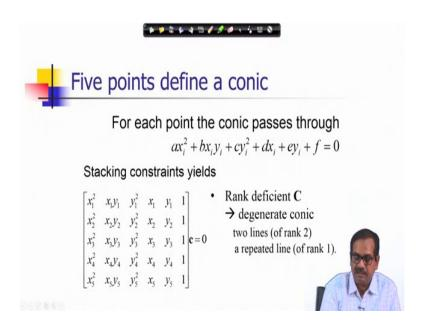
And if I get the five points, I can write five equations and then I can solve this equations because there is a 5 degree of freedom by taking one of the parameter by fixing it at some value, I can solve it. There could be rank deficiency in this representation rank deficiency in
