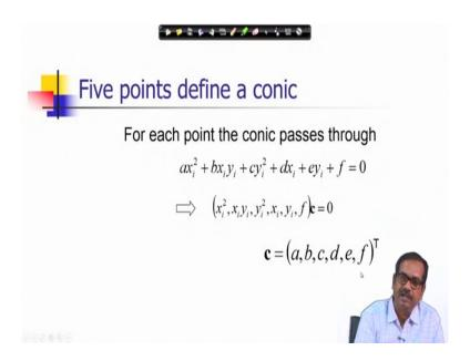
So, naturally to define a conic uniquely I need at least five points in the two-dimensional projective space and I can write those equations using that five points. So, this is the equation, they should satisfy this equation, and this is a representation of a conic also in a vectorial form.
