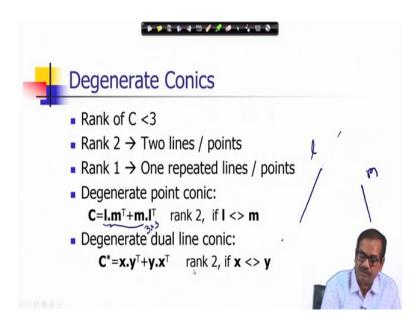
And degenerate conics we mentioned earlier if the rank of matrix C itself is less than 3, then we have some degenerate conditions of representation. Like with rank 2, a conic is defined by only two lines or two points, which are contained in a conic and they are defined only that lines and points. For example, a rank 1 it is the repeated lines and points.
