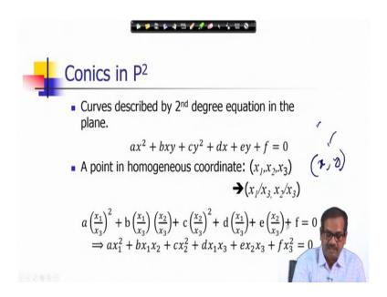
There are there is another element in the two-dimensional projective space which is called conics, which are conics. And we will be considering their representation also in a projective space. So, how conics are represented? They are curves described by secondary equation. And this is the form of the equation which has been shown here.
