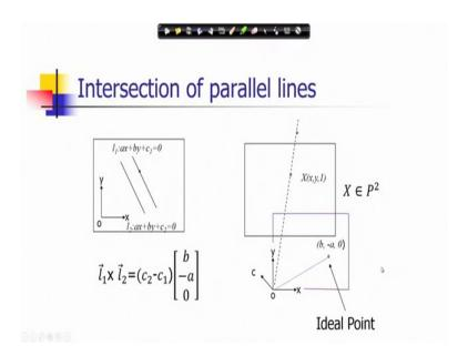
So, if I rub this you know computations, so you can see that we have the point of intersections in this form. And how this line is represented here, this line this particular point of intersection, how it is represented? So, we will say that in the two-dimensional projective space this point b minus a 0 it is represented as a point in a plane which is parallel to the
