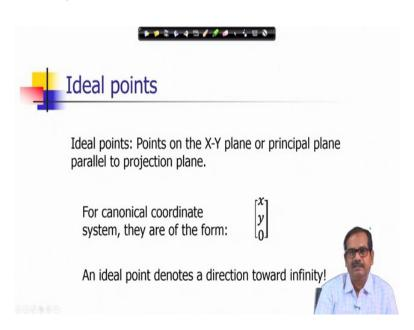
So, just to summarize this fact, ideal points are points on the x y plane or principal plane parallel to projection plane. And for canonical coordinate system, they are of the form x y 0. So, the third dimension which represent the scale that would be 0. An ideal point denotes a direction toward infinity that is the implication of an ideal point.
