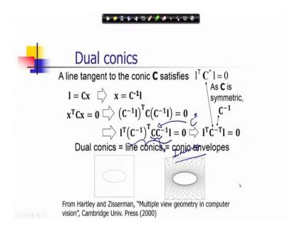
Now, this gives an interesting relationship of a conic representation, we have a dual representation of a conic. In this case a conic can be represented by all tangential lines which is enveloping which forms an envelope of the conic. And you can see that the expression is also in the similar form in the previous case it was x transpose C l, now it is l transpose another representation of conic C star it is a different matrix 3 cross 3 matrix, and l transpose C star l equals 0.
