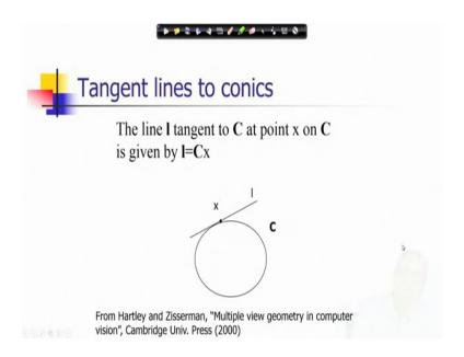
For a conic, its tangent lines are well related very in a convenient from it is related with the point which is lying on that conic, and this is a relationship that is given by simple linear relationships. If I multiply the point with the matrix C, then we will get the corresponding tangent line l.
