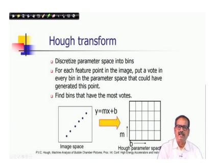
So, these are the operations which are needed when you perform this particular computations. First thing, we have to discretize the parameter space into bins, because in they continuously are from the continuous domain, but in your computations you have to discretize them, so that you can accumulate votes for each discretized cells.
