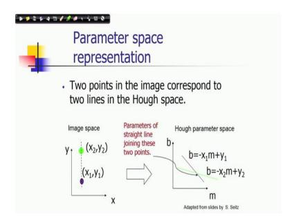
Consider another point (x2, y2) and that would also give you another straight line in the Hough parameter space which has been shown here for the green points I have shown the straight line with green colour which is given by b = -x2m + y2.
