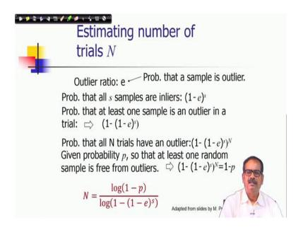
So, one particular issue I will be discussing in details here, that how to estimate the number of trials, how it is related with this outlier ratio e and that indicates what the probability that a sample is outlier is. So, I can make probabilistic analysis in this way.
