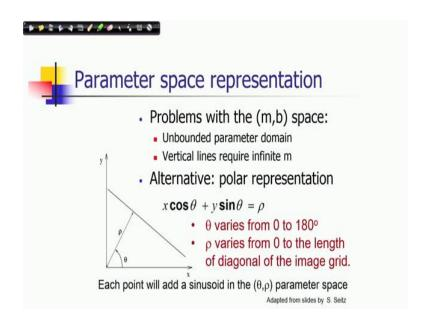
So, there are some problems with this parametric space representation. So, in we are discretizing m and b, because the values of ranges of m and b, they are bit unbounded, so particularly for m. And vertical lines require infinite m there is a problem. So, there are other representations of straight line which is more convenient like polar representation which is given in this form.
