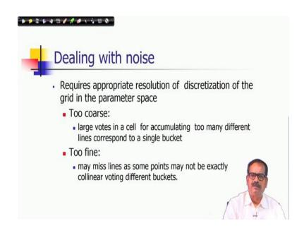
So, these are some situations and one of the major problem or major issue in applying of transform that is it how to deal with noise. In that case, you should require an appropriate resolution of discretization of the grid because if you have two coarse grid in the parametric space then large votes in a cell for accumulating too many different lines correspond to a single bucket. If it is too fine, then you a miss lines as some points may not be exactly collinear and voting different buckets.
