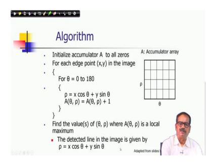
So, the algorithm would be like this that now you consider the discretized space of parameters  $\rho$  and  $\theta$  which is represented by an array here all the cells of an array and let us considered name that array as an accumulated array.
