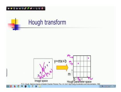
So, let me describe this particular technique with respect to line fitting using Hough transform which follows this approach. You consider a set of points which has been shown here in the image space by circular dots and as we can understand that in fact, there is a straight line passing through these dots.
