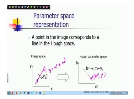
So, this will be explaining further. So, as I was telling that how straight line in the image corresponds to a point in Hough space. So, in the image if you have a straight line as it is shown here y = m1x + b1, you know that exactly it can be represented by a point in the Hough space by (m1, b1). We assume that it is it is corresponding to some discretize bin of m n.
