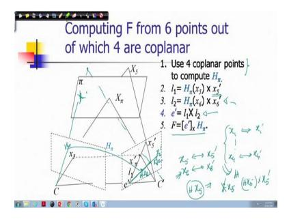
So, we will be considering; we will be exploiting this facts for estimating the fundamental matrix under certain constraint scenarios because that would simplify the computations. Suppose, you would like to compute fundamental matrix from 6 points; out of which 4 are
