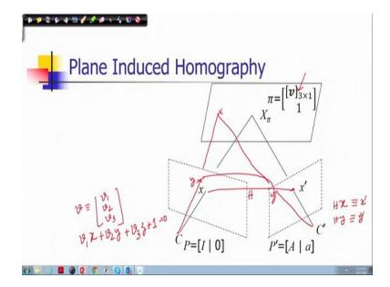
Now, we will be discussing a very important property of a stereo system; an important feature of a stereo system. And you can show that how the projective transformations among the image points they exist in a stereo geometry. So, the homography or the projective transformation are established among the pair of corresponding points for which the scene points lie on a particular plane. So, we call this kind of homography a plane induced homography.
