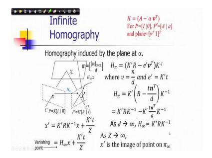
So, these are the things; so v should be equal to n d and e prime is K prime t; e prime is K prime t from here; so that is what is e prime. And then H pi following this you know formulation can be written in this form. So, you note that v is given this n d; so it is t n transpose d. So, finally, it is K prime R K inverse minus this. So, now as d tends to infinity H infinity is K prime R K inverse.
