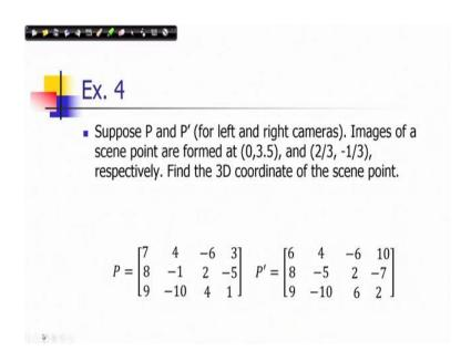
So, consider this particular example that you have two camera matrices P and P' for left and right cameras. And its images of a scene point are formed at say (0, 3.5) and (2/3, -1/3). So, we have to compute the 3D coordinates of the scene point. You can see the projection matrices of the two cameras P and P' they are also given here.
