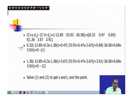
And then we are trying to solve for s and t by applying the constraint that the line forms by this; so the line forms by them this segment it is perpendicular to both the directions of dx and dy'.
