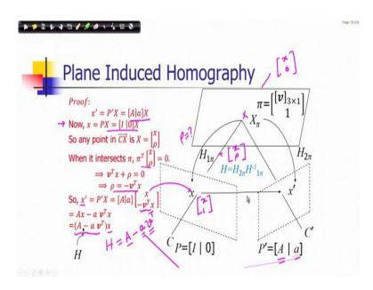
So, we can see that; we have already discussed earlier also that points in a plane and its corresponding image points in a single vis[ion]- camera also they are related by the homography. Because points in a plane can be represented by a three vector by two independent parameters and they are related by a homography; consider that homography is H 1 pi. Similarly, you can have an homography H 2 pi; so from there you can get a homography which is given by this H 2 pi; H 1 pi inverse.
