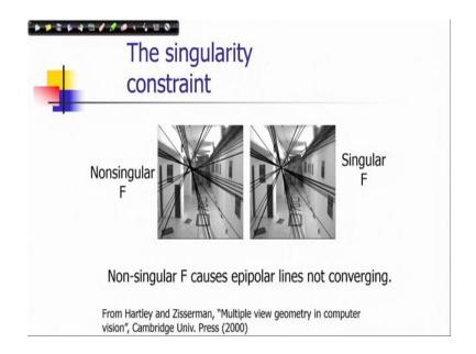
So, one of the nice example that I could get from the book of you know Hartley and Zisserman that is "Multiple view geometry in computer vision". You can see there are the effect of singular F and non-singular F by showing how epipolar lines behave in a particular image plane. So, this is a right image plane with respect to a left image plane which is a reference plane and we are drawing the epipolar lines of all the points corresponding points of the left image planes in the right image plane.
