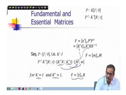
So, if this is a reference camera with respect to this camera, if the fundamental matrix is F, if I consider the other camera is reference camera, then the fundamental matrix will be
