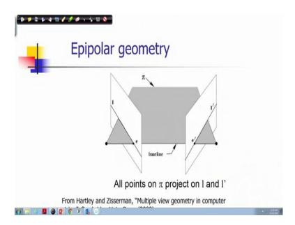
And you can also on interpret this configuration in this fashion also for any epipolar plane  $\pi$ , its point of intersections are those two; its line of intersections with respect to image plane. Those are the corresponding epipolar line. So, all points on  $\pi$  the project on those lines only. So, any point on plane  $\pi$  will be projected for image for the first camera will be projected on l; epipolar line l and for the second camera, it will be projected on epipolar line l'.
