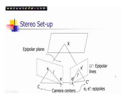
And scene point X for which you will be taking the images in both this cameras. So, if I apply the rule of projection here. So, we get the image of this scene point X in the first camera, whose camera center is given as C as a say x.
