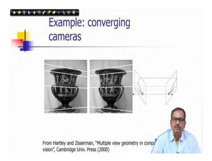
So, typical examples of converging camera images. So, were it is shown that their epipolar lines are converging. So, this is one example, I have taken from the book of Hartley and Zisserman which is also shown here multiple view geometry in computer vision. You can find, you can see that how epipolar lines they can be mapped on those images and you can find out those all those epipolar lines, they are converging in this case.
