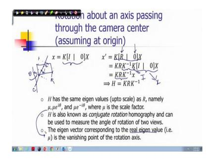
So, right now, what we are going to discuss suppose, the camera center is fixed, but you have rotated the image plane about its vertical axis. So, you consider this scenario that you have an image plane and you consider a center C and there is an image formed in this plane which is given by x.
