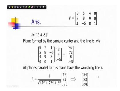
So, all planes parallel to this plane have the vanishing line l. So, that is the interpretation and the normal can be computed in this fashion. So, we can finally, we can compute the normal as we can see into this computation.
