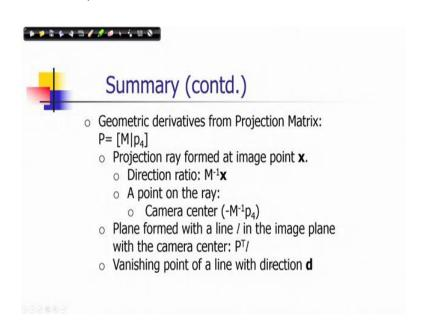
So, there are different other geometric derivatives from projection matrix. First thing is that you can form a projection ray at an image point, you can from its three dimensional equations of that particular line, it is direction ratio is given by this expression  $M^{-1}x$ . You note that x is a image which is expressed in the homogenous coordinate system of a 2 dimensional projective space.
