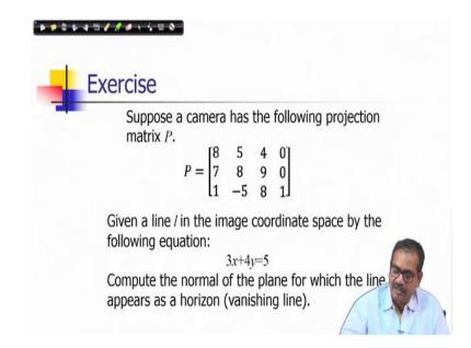
So, let us again workout an exercise for involving this particular computation. Suppose, you have a camera which has this following projection matrix that is P which is given here as you can see, and suppose you have a line in the image coordinates space by the equation 3x + 4y = 5. So, we have to compute the normal of the plane for which the line appears as a horizon. So, you understand your horizon should be the vanishing line of that plane which is the parallel to our particular view.
