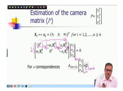
So, this is the summary finally, as you can see I have eliminated the third row just to show that there are only two equations which are formed by using a single point correspondence. So, if I have n such points, n point correspondences each one will give me two equations. So, I will get 2n such rows for n point correspondences and what is the dimension, if I note the dimension see each one is it is a  $1\times3$
