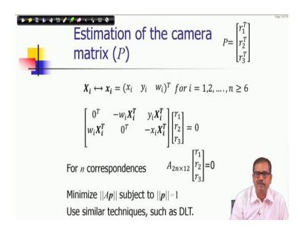
So, the as you understand that you have more number of equations than the number of unknowns so, you have to apply a least square error technique what we did earlier for estimation of homography also and in this case, it is a set of homogeneous equations these linear equations they form a set of homogeneous linear equations.
