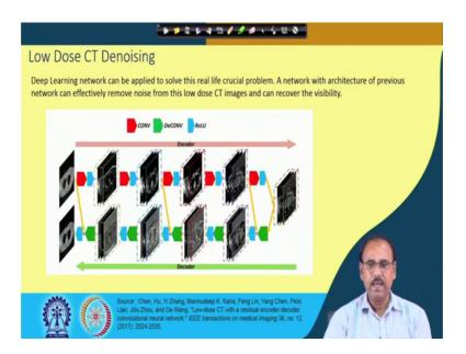
And once the network is trained and this is the architecture of the network that can be used for this denoisy purpose; denoising purpose, which is same as that skip connection network.
