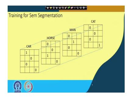
So, let us see that what is dice loss and before coming to that, let me just recapitulate that what is an array of one odd vectors and how using this array of one odd vectors, we have computed the pixel wise entropy loss. So, the array of one odd vectors is something like this, that your output array is of the same size as that of the input image.
