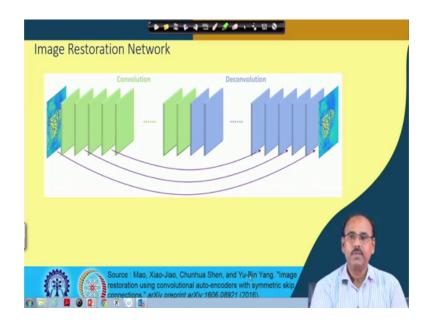
So, let us see how we can do it. So, a neural network which has been suggested as suggested by the authors of this paper, which is on image distortion network. So, this image distortion network, it is a deconvolution network, where I have arrays of the convolution networks followed by an arrays of a set of deconvolution networks. And this particular network, the deconvolution network also makes use that the concept of the skip connection.
