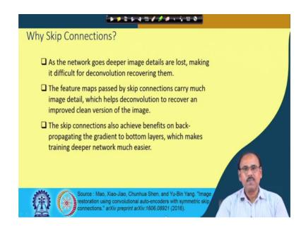
So, let us see over here; what this skip connection does. As we have seen that because the skip connection, output of a convolution layer is directly added to a deconvolution layer, the corresponding deconvolution layer. The convolution layers, which are in the shallower part, for them the removal of the detailed information of the image will not be that severe. But, as you move inside the deeper layers, the detailed information will be lost more and more.
