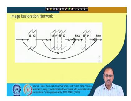
Now, when you have this deconvolution network, the authors of these papers, they have suggested the architecture of the image restoration network or the block of the image restoration network is something like this. So, you find that I have a deconvolution layer say d 4 and the corresponding convolution layer is c 1. Corresponding to c 1 which is a convolution layer, I have the corresponding deconvolution layer d 3.
