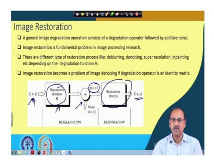
Any image capturing operation, follows through I mean goes to this degradation steps. So, suppose my actual input image is f x, y. This f x, y goes to a degradation function, which is H as shown over here. So, I have my actual original input image, which is H there is a degradation operator and after degradation operator I have an additive noise. So, at the output of this block, I get an image g x, y, which is degraded and noisiness.
