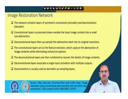
Now, what does this convolution layers and the deconvolution layers that actually do. You find that in this particular case, the convolution and deconvolution they have mirror symmetry right. The number of convolution layers and the number of deconvolution layers they are same. The way it is reduced on the convolution side, just in the inverse way the size is increased in the deconvolution side.
