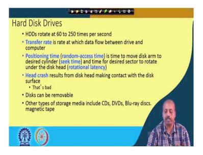
So, this hard disk drives they rotate at 60 to 250 times per second and transfer rate is the rate at which data flows between drive and computer. So, that is the transfer rate the rate at which the data can move between the computer and the drive.
