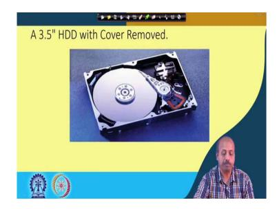
So, this is how a disk drive looks like. So, this is your disk ok. So, and this is the read write assembly, the head assembly. So, as you are giving pulses to this read write head, so it can go move from one cylinder to the next cylinder. So, it can move like this and this head this disk can move this and as a result the corresponding sector will come below the read write head from where it will be able to start doing the read operation.
