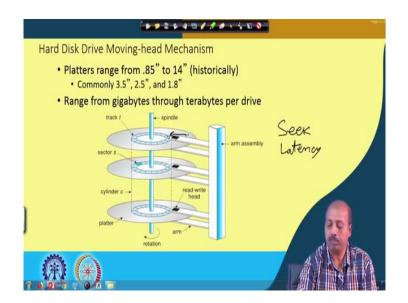
And then I need to access this particular cylinder, then this disk head has to move by this much amount and that is done by a mechanical motor and an electrical motor.
