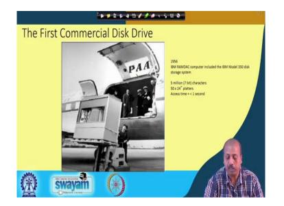
So, this is the first commercial disk drive. So, that was in 1956 IBM computer, RAMDAC computer is included the IBM model 350 disks storage 5 million characters. Each character is 7 bit.
