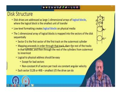
Coming to the structure of disk : so, disk drives are addressed as large one dimensional array of logical blocks as I said that unlike primary storage. secondary storage is not accessed in terms of bytes or words. So, they are accessed it in terms of blocks and one
