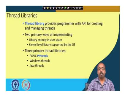
Now, going to thread libraries; so, they there are different libraries that have been created for helping the user to write programs using the using this threading philosophy. So, otherwise will be it is difficult to develop applications around thread using this thread concept, with thread library it provides the programmer with an application API interface for creating the creating and managing threads.
