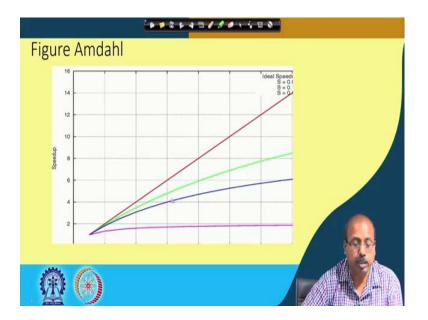
So, next we will have a look at a graph that shows that ok. So, this is the ideal situation. So, as you are increasing number of processors, then the speed up should grow like this. So, this redline so, with 1 the speed up is 1 with 2 the speed up should be 2 with 4 the speed up should be 4.
