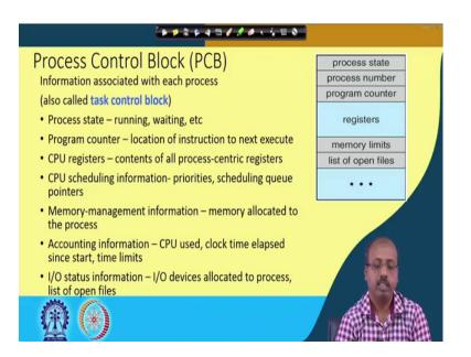
So, every process has got a control block associated with it which is known as the PCB or the Process Control Block. So, here we note down all the important information about the process. So, information associated with each process so, they are stored in this process control block or task control block.
