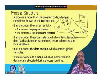
The structure of a process a process is more than the program code which is sometimes known as the text part. So, it also includes the current activity which is the program counter and the contents of processor registers. Also includes process stack which contains temporary data and the data section which has got global variables and it has got some local variables in the some dynamically created local variables in the heap.
