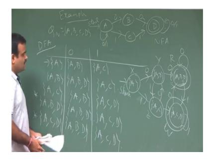
So, if you do that we can just construct the DFA. So, this is A 0 1, 0 1. So, from A so what we do from A we can go to B and C. So, this B and C with the 0 move know with the 0 move we can go to B and A. So, this is A B will write and now with 1 we can only go to. So, 1 we can go to A and C.
