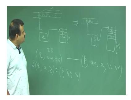
Like if we have if our control is like this, we are reading a tape like this. So, we have a, a 1, a 2 and this is the current tape header. And we are at state q and this is the stack position, we have some symbols say top is z, this is z 1, z 2 dot dot dot ok. And suppose it is so this is the control unit this is pointing this a and it is pointing the top of the head. So, this is the current ID.
