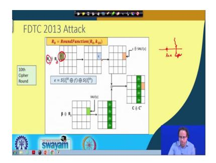
So, let us see you know like how that works and here is a depiction of the how that works. So, as you can see that the fault is in the 10th cipher round. So, R 0 is equal to round function R 0 comma k 10 and here is the fault. The fault has been shown over here as this is the first byte of the second row and that has been faulted by value and so, showed here as f.
