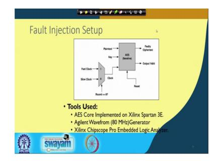
So, again this is our fault injection set up again it is kind of similar to what we have done previously. So, we have got the AES iterative hardware implemented and we are again kind of tinkering with the clock line ok, so we can again try to induce the fault in other mechanisms.
