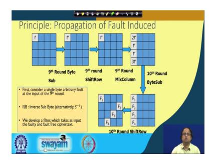
So, now let us try to see how the fault propagates. In particular just to understand the principle let us consider AES 128 where the fault as we induced on the input of the 9th round.
