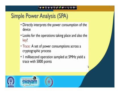
So, therefore, we have already studied that in SPA, right. We basically work with like maybe 1 trace or may be 2 trace or may few 100 traces. And the trace is nothing but a set of power consumption across cryptographic operations like when we take we will be execute the cryptographic process, right, we are basically trying to measure the power consumed of the total device.
