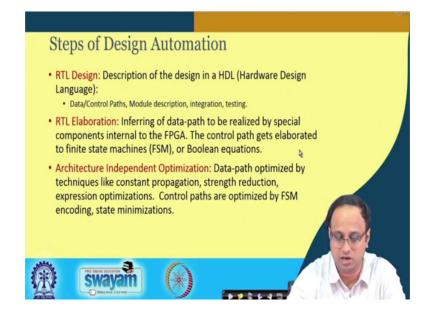
And, automatically your tool will go through a bunch of steps, ok. And, these steps essentially I have got several important components. So, first important component is that it does and RTL design as a like you already done this RTL design. Once you have done these you know like the next step which is done is what is called as an RTL elaboration.
