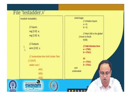
So, if you see the test bench right I mean again without going into the syntax, you basically instantiate the adder which means you kind of scan sane inputs to the adder. And the input sequence is denoted here. So, you are basically giving stimuli to your adder. So, you are giving say 0 0 as an input or a 1 1 or 1 3 as input and so on.
