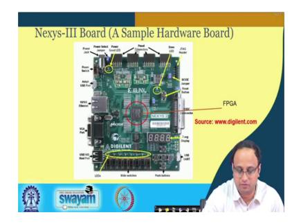
So, this is how the overall design flow looks like and what I will try to you know like show you was one of the sample boards which you can probably try to get access to. Is a relatively low cost FPGA device which is a called as an Nexys-III board and you know like we can actually. So, this is the FPGA inside the board and what we will be trying to do is we will be trying to program this FPGA using our design and typically and reconfigure it to work as we want.
