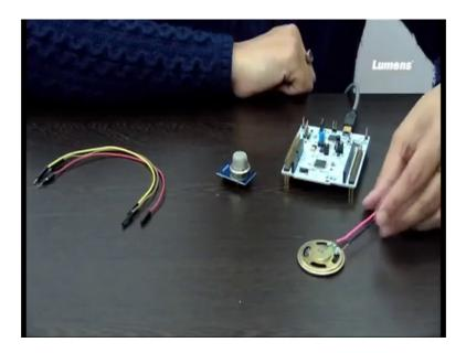
So, this connection I will make and this is the speaker the speaker I will be connecting one to ground and another to one of the PWM port. In this case we have used D 3 port as the PWM port ok. So, let us first make the connection.
