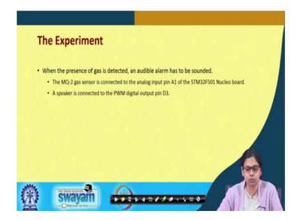
So, in this experiment what we will be doing when there is a presence of gas, then an audible alarm will be activated ok. So, the MQ2 gas sensor is connected to the analog input pin A 1 of STM board and a speaker is connected to the PWM output pin D3. There are other PWM output pin as well, but we have connected it to PWM digital output pin D 3.
