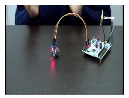
So, first one is BCC. The next one is ground, next one is ground and then the last one is that analog which I will be connecting with the a 1 pin of STM ok. This is a simple
