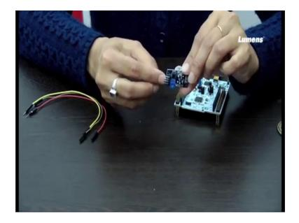
This is the gas sensor that we will be using. You can see there are four pins that are connected ok. So, what are those pins? One is AD; another is DD, another is your ground and another is your BCC ok. These are the four pins. So, I will be connecting the ground the BCC and I will be taking the analog output ok. So, I am not concerned about the digital output, I am concerned more about the analog output. So, I will be taking the
