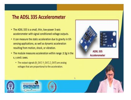
Now, the accelerometer that we will be using in this experiment is ADXL 335 accelerometer, where you can see that these are the pins of this accelerometer basically. You have this V CC; we have this ground; and we have x, y and z coordinate. So, this is from the other side and this is from the other one. So, this arrow shows the x axis, this arrow shows the y direction, and this one is the z one, z direction.
