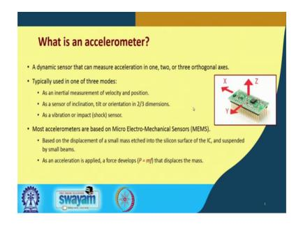
So, what is an accelerometer? It is defined as a dynamic sensor that can measure acceleration in one, two, or three orthogonal axes that is X, Y and Z. And typically it is used in one of the three modes. It can be used as an inertial measurement of velocity and position. It can be also used as a sensor of inclination, tilt, or orientation in 2 to 3 dimensions, or it can also used as a vibration or impact sensor, shock sensor that we see.
