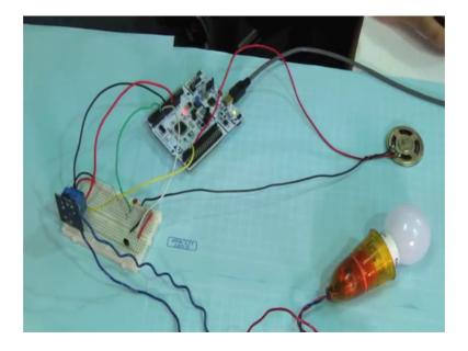
Now, let us come to this circuit now see we have used that same light interfacing circuitry as was shown earlier a relay a bulb with a switch connected to mains and we have used the same LDR circuit you see if LDR is interrupted, the light is glowing if LDR is interrupted the light will glow. You see if it is released again light will and here you have this LM35 setting here; if LM35 temperature exceeds the threshold, but as I
