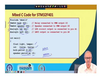
The program will start like this. So, you are defining a PW outline on D3 which you call as bulb then another PWM out on D6 which you call speaker and there were two analog inputs one on A 1 A 0 corresponding to LDR and lm thirty five.
