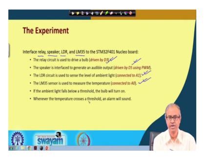
So, specifically in this experiment as it said will be interfacing a relay per speaker and LDR and LM35 and these specific ports that will be using the relay will be driven by digital port line D3. This speaker will be interfaced from port line D5 the LDR circuit the output of it will be connected to the analog input A 1 and the LM35 sensor will be connected to analog input a 0.
