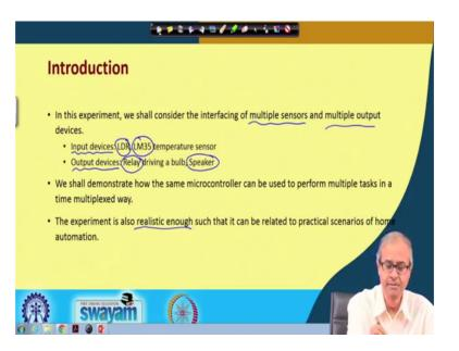
Let us talk about the experiment first now in this experiment as it said we shall be interfacing multiple sensors and multiple output devices; specifically the input devices that we shall be looking at are LDR for sensing ambient light and a temperature sensor for sensing the temperature of the environment.
