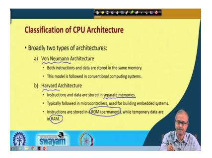
Broadly with respect to CPU architectures we are so far talking about instruction set architectures, now talking about how the CPU works there is a broad classification here also we talk about Von Neumann and Harvard class of Architectures. The basic difference is that in the Von Neumann Architecture we have a single memory both instructions and data they are stored in the same memory, most of the conventional computer systems that you see around us they are based on Von Neumann Architecture ok.
