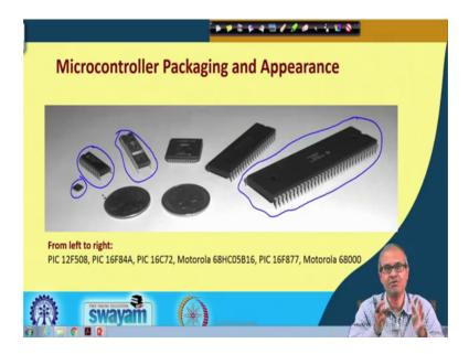
Microcontroller packaging and appearance you can see these are some typical microcontroller which are manufactured by a company called PIC, PIC microcontrollers. Now, in comparison you see one of the older micro processors Motorola 68000. This was a 48 pin chip, so large in size. So, in comparison the smallest PIC processor is so small, it is a fraction of the size of a coin as you can see.
