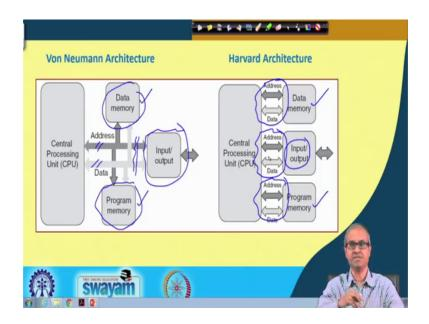
Pictorially for Von Neumann Harvard Architectures can be shown like this. In a Von Neumann Architecture as you can see here the data and program memory although you are showing them as separate, but CPU is accessing them over the same data bus using the same address.
