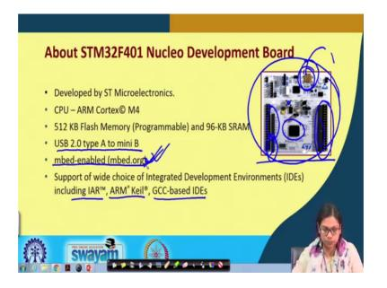
Now, I will move on with STM 32 F 401 nucleo development board, this is the board this is the board which we will be using it has got some digital pins it has got some analog pins, there is a power thing this is the USB connection through which you can connect through USB. So, let me talk about a little bit about this board.
