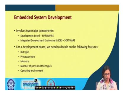
Embedded system development; when we talk about this embedded system development this involves two major components; what are those? One is the development board that is the hardware that is required and another is Integrated Development Environment, we call it IDE that is the SOFTWARE.
