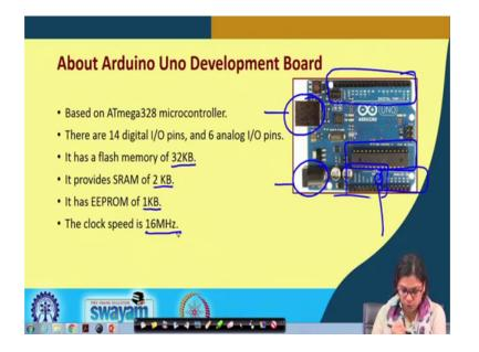
Let us now move on and I will be discussing about this Arduino UNO development board. So, this is the Arduino UNO development board you can see these are the digital and PWM ports this is the analog ports, this is for the power, this is the microcontroller chip that is there. You can use the USB connector to power it or you can also use this you can use through this 9 volt battery to power it and there is also another one here, sorry this v in basically it can be used to power it.
