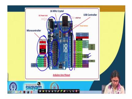
Now, let us move on this is the broad diagram. So, as I have told you this is the USB port through which you can connect to the USB port of the PC. This is the microcontroller that we are using these are the analog pins set of analog pins, these are for the power. And if you see these are digital pins, but some of the digital pins are also PWM, we will look into this specifically what is PWM?
