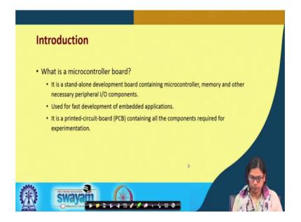
So, let me talk about what is a microcontroller board? We can define it as a standalone development board containing microcontroller, memory and other necessary peripheral I O components. Why it is used basically? It is used for fast development of embedded applications. And, it is generally built on a printed circuit board which is called PCB containing all the components that are required for the experimentation.
