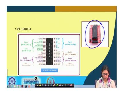
PIC board typically consists of these pins and these are some typical features this is port A; port A is from pin number 2 to pin number 7 port E is from pin number 8 to 10 and port C is there port B port D and port C. So, each of the pin has got certain functionalities and there are various features of this particular pin. So, this is a sample diagram showing PIC 16F877A microcontroller this is how it typically looks like ok.
