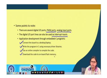
Now, at this point there are some points to note as we know there are several digital IO ports there are also PWM Ports pulse Width Modulation enabled boards and there are analog input ports. The digital I O port lines can be used as interrupt inputs as well this is already discussed in more detail it will be discussed later and for application development through embedded C programs what needs to be done you need to connect the board to a desktop or a laptop that we will be doing ok.
