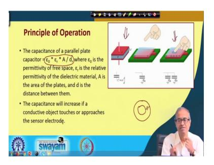
Now here as a very short explanation is given. This diagram here shows how a parallel plate capacitor looks like. There is a plate whose area is A, there are two plates parallel plates the separation is small d and there is a material in between that is called a dielectric, there is a dielectric constant. So, the value of the capacitance is given by this expression epsilon 0 multiplied by epsilon r multiplied by the area A divided by the separation.
