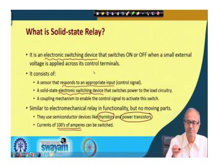
Solid state means everything is built inside a chip semiconductor device.
