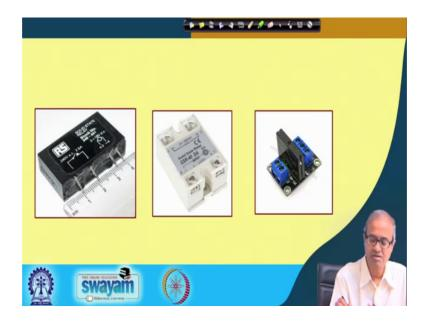
So, this is how solid state relay works. These are some of the pictures of some solid state relays. So, you see this is the middle one, it says that it works from 24 to 380 volts AC. So, there are these are much smaller in size because the semiconductor made of solid state devices, they are much smaller in sizes. So, you can see. So, one on the left you can see the dimension it is out 4 centimeters total in size, this middle one this middle one the same device is been shown here.
