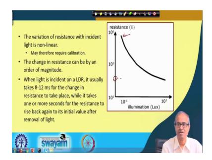
And the other properties, that as the illumination increases the intensity of light well the unit of illumination is Lux you may be knowing. So, as the illumination increases the resistance decreases exponentially. So, one point in notice that you see we unlike LM 35 this is not a linear device the resistance is not proportional to the intensity level it follows this kind of exponential curve.
