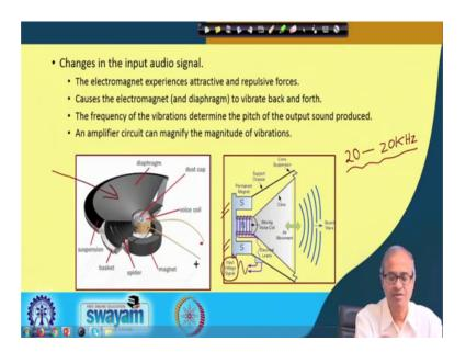
So, just looking into the diagram yes you see I have shown a diagram here the permanent magnet is shown in the back this is the permanent magnet. And in the coil, coil is wound around a middle point this can be connected or attached to the permanent magnet or this can be a separate movable part also there can in two different kind of speakers you can manufacture.
