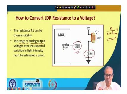
Now, talking about interfacing while interfacing very typically we use some kind of a resistance divider circuit like we can use an LDR we can use a resistance R1 with a 5 volt supply let us say and this we can feed it to one of the analog input pins of our microcontroller either Arduino or STM 32. So, here this voltage output what will be the value it will be this R1 divided by R1 plus resistance of the LDR multiplied by 5 volts this will be the value of this output voltage.
