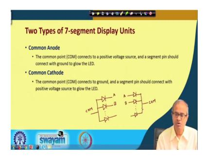
Now, depending on how the light emitting diodes are connected inside these 7 segment display units can be of 2 types either common anode or common cathode, common anode means a inside there are so many LEDs. So, I am showing these LEDs like this, there are 8 LEDs is in total. If the anode terminals are all connected together and this is your common point then we say that this is a common anode kind of our display.
