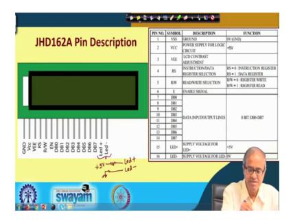
And the last 2 pins this LED plus and LED minus, these are used to control I told you that there is an LED backplane in typical LCD displays, which controls the brightness level. So, you can connect a voltage across LED plus and LED minus to make the display bright typically, what you do with 5 volts, you can connect a resistance, you can connect it to the LED plus input and the other input you are connecting to LED minus, this you can ground, this is how you can connect ok.
