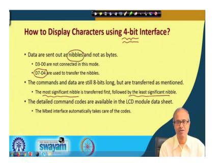
And now talking about the interfacing issue; so, in our experiments because of simplicity, we shall be using the 4 bit mode because, only 4 data lines have to be connected otherwise 8 wires have to be connected ok. Now, I told you in the 4 bit node data are written into the display device, 4 bits at a time, 4 bit is called a nibble byte is 8 bits. So, data are sent as nibbles.
