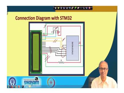
So here, I am showing a very typical interface with the STM microcontroller to this board you see here I am connecting the LED plus and LED minus connections. Here, the first 2 are the power supply and ground you see here, I am using a potentiometer on one side, I am connecting ground on one side, I am connecting 5 volt the middle point, I am connecting to the VEE terminal that is the contrast control.
