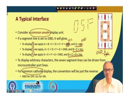
Now, a typical interface like you see when you have a display unit like this let us assume that I have a common anode display common anode means my common terminal is connected to 5 volts, I have connected 5 volts to it and to glow a segment the corresponding segment pin has to be connected to ground 0 volts ok.
