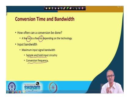
Now conversion time and bandwidth are two other parameters, conversion time is how much time it takes for the AD converter to convert a convert a given input analog voltage into the output, digital equivalent right.
