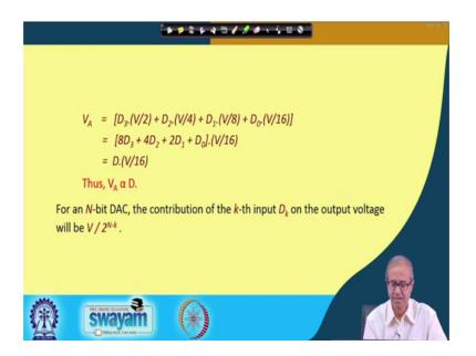
V A is proportional to D. So, for N bit D A converter in general if you look at the k-th bit, the contribution will be V by 2 to the power N minus k in general. So, we checked it for a 4 bit D A converter ok.
