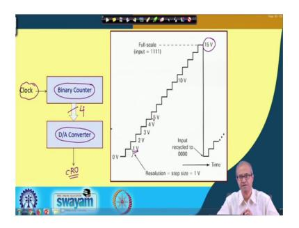
So, let us look at one thing. Suppose we have a DA converter like this and to the input of the DA converter let us say, we have connected the binary counter which counts up and we apply a clock continuously the clock is coming. So, the counter will be counting up 0 1 2 3 4 like that, let us say this is a 4 bit DA converter. So, there are 4 number of lines here and it is a 4 bit counter.
