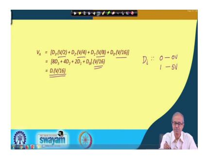
So, you will be getting some expression like this. So, where D 3 will be having a weight in V by 2 we said D 2 into V by 4 D 1 into V by 8 D 0 into V by 16 where this D i is are the digital inputs ok. So, when you are applying 0, this will be 0 volt; when you are applying 1, let us say this will be 5 volts.
