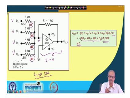
This is how this circuit looks like. So, here I am showing a 4 bit D A converter of weighted register type. So, you see the values where using are R 2R 4R and 8R just as an example I am showing it to be 1 kilo ohm, 2 kilo ohm, 4 kilo ohm and 8 kilo ohm; 4 values and the digital inputs are applied like this D 0 D 1 D 2 D 3 least significant bit is connected to the highest resistance most significant bit is connected to the lowest
