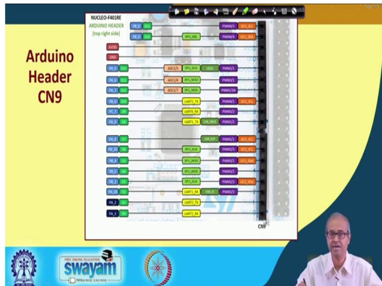
And, the second set of Arduino connectors that appears on the right side that is like this is called CN9 connector that is this is a larger sized connector. This contains many signal as you can see so many pulse width modulated ports PWM you can see there are. So, many I2C ports also some of them you can use, these are USB, UART pins, these are some additional AD converter, these are some is analog input pins and these are some port pins. So, you can also use them as some IO port pins.
