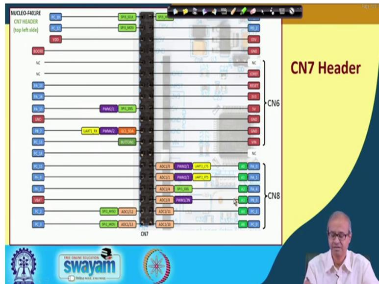
Now, these are the detailed pins that are coming from the microcontroller sitting inside the board. On the left side this is called CN7, this is the big connector those pins you have seen, and here the signals are all mentioned all port Port C, Port A. You see, Port A, Port B, Port C there are three 16-bit ports which are available in the microcontroller. So, all those 48 pins are available over these connectors.
