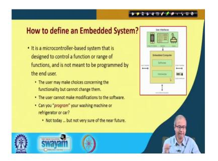
Now, how can we define an embedded system based on whatever we talked about so, far? Well embedded system can be loosely defined as a microcontroller based system. This is true for most of the embedded systems. The processor that is inside I said it has to be low cost it has to be low power, it has to be smaller in size. There is some kind of processor called microcontroller which we shall be talking about throughout this course they satisfy all this criteria.
