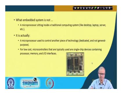
Now, what embedded system is not? Well it is not a microprocessor sitting inside a traditional computing system no it is not. We call it a computer we do not call it an embedded system right. Well it is a microprocessor used to control another piece of technology like SA machine, like microwave like refrigerator and so, on this is what an embedded system is.
