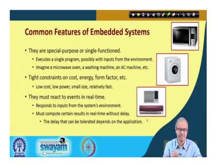
So, there are some common features which are present in most embedded systems let us look at some of them. First thing is that, they are special purpose or single functioned single functional. Like an air conditioning machine, there is a processor inside, the sole purpose of that processor is to ensure that the ac machine is working properly nothing else. So, it is not trying to help you in calculation in doing some maths and so, on.
