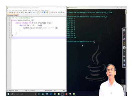
Now, similar to while and do while there is another constructor in Java it is called the for loop. For loop is totally different than the while loop or do while loop. Now, in case of any loop there are three things are to be considered initialization for the loop variable, in the first two examples the loop variable was count.
