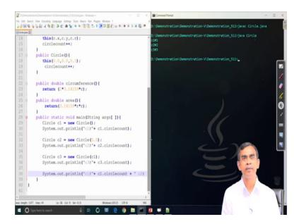
So, here each circle of object is created once the circle object is created the static variable will be processed according to the objects construction and then it will basically run the it will print the current value of this one. And here we can understand that the circle count is a global variable look like for all instances of the objects there is only 1 instances of this variable. So, here we can see the running of the output is basically 1 2 3.
