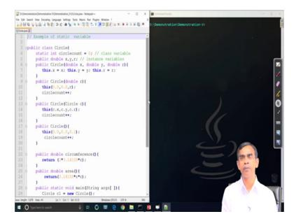
However the concept of global variable is by means of the concept of class variable; a class variable and then instance variable as we have already learnt about it. Here for example, x y r these are the instance variable because they are declared as simple as a type; on the other hand if we declare a variable with a skiver static then it is called the class variable, in this case we can see the circle count is an example of a class variable.
