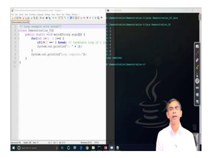
So, this is idea about the continue like continue there is one break statement; the break statement whenever a condition reaches. So, it is basically terminate the loop without any satisfaction of the loop control termination criteria. So, this is example here we can see here i mode 10 indicates that whenever the value of i reaches to 10 or multiple of 10 whatever it is there so, the loop will be terminated.
