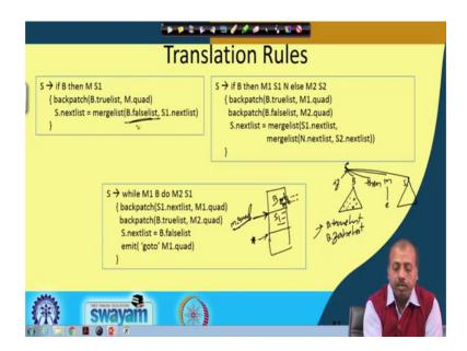
So, first one; so, if the if then statement, so, if B then MS1. So, what we will have to do is that. So, so, in this particular reduction is being made you see that I have got this situation if B then M and S1. So, by this time this B has already been reduced and we have got with associated with this B we have got B dot true list and B dot false list.
