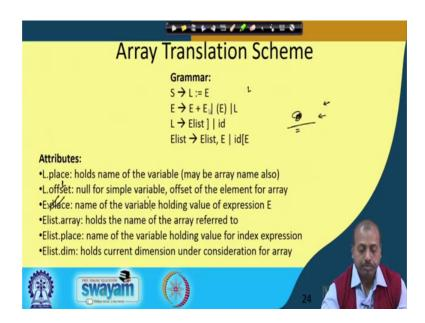
So, this L dot place it holds the sorry Elist dot place is the variable holding the value for the index expression, at any point this whenever it is done so, L producing Eist. So, L should so, L dot place should hold the name of the variable, which may be an array and L dot offset will be the offset within the within the array.
