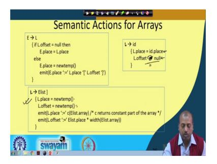
So, the next rule that we have for the array reference is this L producing i d. So, for this L producing i d the situation is very simple. So, this L dot place. So, this means that that L that I am talking about it is a single variable it is not an array.
