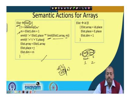
So, now if I multidimensional array. So, I will have to do it like this that Elist producing Elist 1, comma E. So; however, so, then this t equal to newtemp. So, this gives me a new temporary variable. And, m so, this holds that this is the new dimension that I that I have got. So, Elist 1 dot dimension. So, that was the dimension that we are considering previously so, which was this part.
