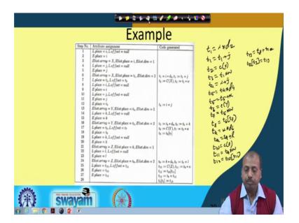
So, this is the action that goes on as we proceed through this parse tree and try to generate the code. So, at step number 1 so, at step number 1 is this one. So, this L producing i d and the rule for that is L producing i d. So, L dot place is i d dot place L dot offset is null.
