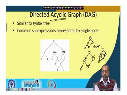
So, the previous representation that we had that was a tree. So, syntax tree and now this is a graph and you know that as a data structure the difference between tree and graph is that, in case of tree every node has got a unique parent node. And one so, it so that parent is only one every node has got at most one parent the root node does not have any parent, but otherwise like if this is a tree. So, the tree is always like this.
