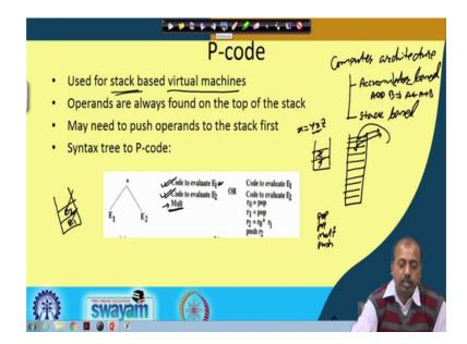
Then there is another high level representation which is known as P code. So, this is used for stack based virtual machines. So, what is a stack based virtual machines? So, virtual machine means the machine does not exist in actual ok. So, this is a conceptual machine you can say may be there are some machines which are built around this concept, but it is, but the basic idea is that this is a stack based machine.
