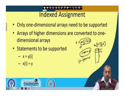
So, it will do that conversion and so, I like I can have definitely have a statement in my source language program like say t equal to say x i j. And then in the three address code I should have the appropriate code so, that this x i j so this is converted into some one dimensional array.
