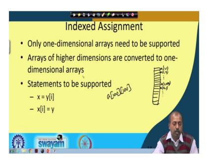
So, it also supports some array type of structure because array is now so, common in most in many of the almost all the programming languages. So, if you do not support array as a basic operation in the three address code, then it becomes very difficult to generate the corresponding code in the target machine. So, or so it becomes very difficult for converting the source language array indices to the intermediate code, so, only one dimensional array is supported.
