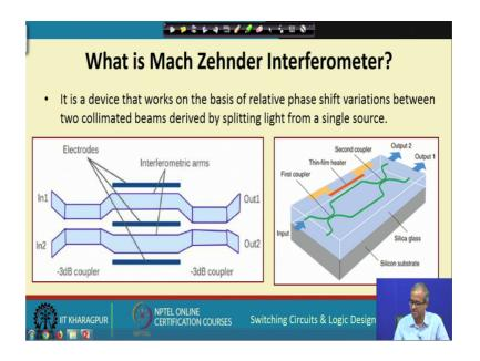
Here we have a very high level schematic diagram of a Mach-Zehnder Interferometer. As you can see it is a device which works on the basis of relative phase shift of 2 beams of light. As you can see in this diagram on the left there are 2 paths which are shown one is wire here other is wire here.
