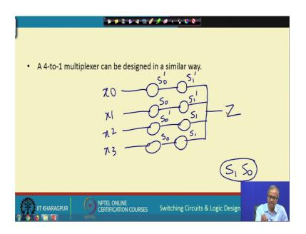
So, using transmission gates it is very easy to do so, you can have a 4 to 1 multiplexer in the same way, I am not showing with the complete diagram, just giving you an idea suppose my four inputs are x 0, x 1, x 2 and x 3 and each of these lines I connect 2 such switches, 2 such transmission gates I am showing it as a circle like this, and the outputs I connect together let us say I call it z this is the output.
