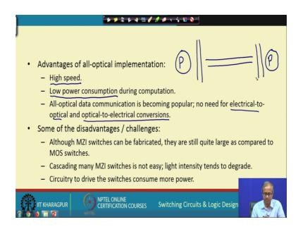
So, some of the advantages here, because light is very fast you can have high speed computation. Power consumption will be low, because everything is depending on the flow of light only no other circuits are required and because we are already doing communication. So, electrical to optical and optical to electrical conversions are not required if you are can do everything in optical.
