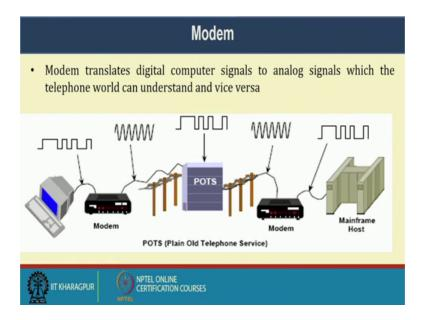
Now if you look at the modem, modem translate the digital computer signal to analog signal which is the telecom network or the telephone backbone understands and carry it
