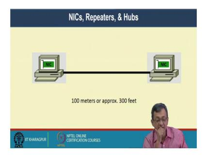
So, typically this cable can be stretched up to 100 metres or 300 feet that for say fully construction of things, but in reality we may not able to go that path it is little less than the 100 metres considered as a, otherwise signal degradation will be much higher to handle that.
