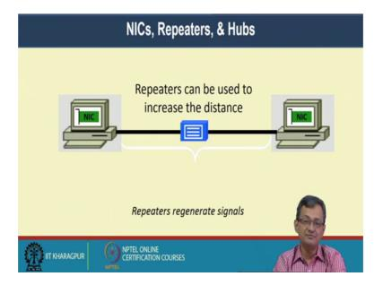
If it is more then we require something call every repeater right. So, a repeater which regenerates the signal right so that is a repeater can be used to increase the distance. So, if I have repeater, again the distance is increase there right. So, repeater regenerates the signal.
