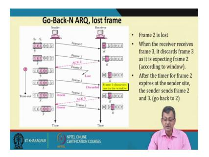
And in case of a lost frame. Frame say in this case, frame 2 is lost, when the receiver receives frame 3 discards frame 3, it is expecting 2 as we are discussing. So, it has expecting, 2 here and receive 3 instead of 2 discards. The timer from the 2 expire and the sender side and sender sends frame 2 and 3, go back to N, that is go back to 2, in this case.
