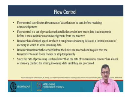
So, flow control coordinates amount of the data that can be sent before receiving the acknowledgement right.
