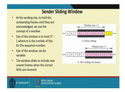
So, from the sending send the sliding window at the sending a to hold the outstanding frames, until they are acknowledged, we use the concept of a window right, because unless this is acknowledged that has to hold right. We cannot discards those that the sender ends, size of the window is at most 2 the power of m minus 1, where m is the number of bits in the sequence number right.
