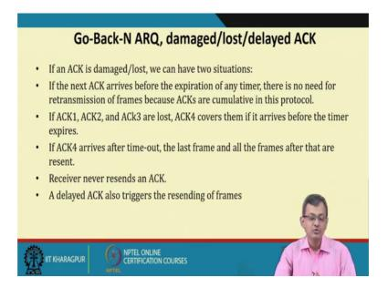
Go back to Go-Back-N ARQ damage, lost, delayed acknowledgement. If the acknowledgement is damaged or lost, we can have 2 situations, if the next
