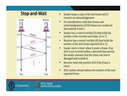
So, in case of stop and wait it is pretty straight forward, sender keeps a copy of the last frame, until it receives a acknowledgement right. So, sender keeps a things for the identification both frames and the acknowledgment are numbered alternatively 0 and 1 so, 01, 01 and type of things right. So, once the frame is sender the 0, acknowledgement comes as a 1 sender frame as 1 acknowledgement comes as 0 and alternatively goes on right.
