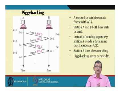
There is a concept of Piggybacking right. Now because, this both sending the data and acknowledgement are eating away space. So, when we have a both communication, both side communication like station AB, both have data to send then the a method to combine data frame with acknowledgement, the data frame itself carry the acknowledgement.
