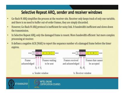
Selective ARQ sender and receiver windows, this is another ARQ mechanisms. So, Go-Back-N ARQ simplifies process of the receiver size right, receiver only keeps track of only 1 variable right and there is no need of buffer out of order frames and simply discard the things, if anything out of the frame coming, in case of a Go-Back-N ARQ.
