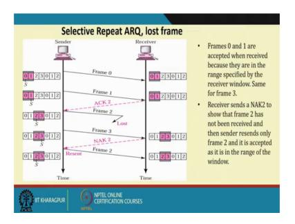
So, in selective repeat ARQ, lost frame 0 and 1 are accepted, when the received accepted when receive because, they are in the range specified by the receiver window of the frame (Refer Time: 26:47).
