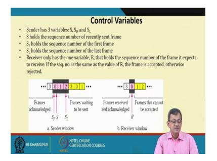
Control variable, sender has 3 variable S, SF and SL. So, 1 is the end of Markats that is what we say first frame, last frame and S is the currently send frame. So, right receiver has only 1 variable R to hold the sequence number of the frame, it expects to receive. So, it is expecting 0 to receive it will be on that things, if the sequence number is the same as the value of R.
