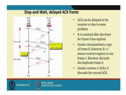
Stop and wait, delayed acknowledgement frame. So, happen that acknowledgement is same, but it is delayed right acknowledgement can be delayed at the receiver or due to some problem right. It is received after the timer for the frame 0 has expired sender transmitted a copy of the frame 0; however, R equal to 1 means, the receiver expect to see a frame 1 right. So, receiver discards the duplicate frame 0 right. The previously what to was there?
