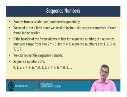
So, as we bunch of frame, there is not 1 sending and receiving and type of thing. So in this case, what we require is a sequence number right, frames from a sender are numbered sequentially, we need to set the limit since, we need to include the sequence number of each frame in the header, set a limit. So, if the header frame allows m bits for the sequence number.
