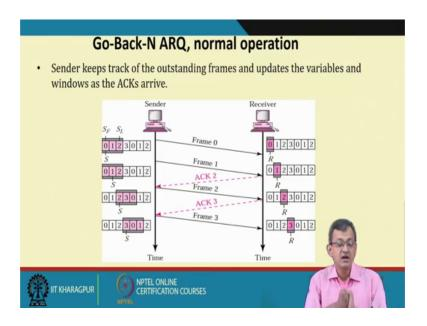
So, this is the Go-Back-N ARQ, sender keeps track of the outstanding frames that are an updates the variables and windows at the acknowledge arrives right.
