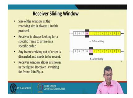
At the receiving window, size of the receiving window is always 1 for this protocol right. Receiving is always looking for a specific frame to arrive in the specific order. So, whether it is sliding or not at the sender end, receiving is waiting for that specific number of frames, may be in the sequence to wait for the in a specified order right.
