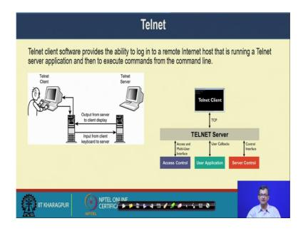
There is another protocol which is called Telnet, right. So, that which allows me which allows us to connect to a remote system or site. So, Telnet client provides ability to log into a remote internet host that is running a Telnet server. So, any client should have a corresponding server at the other end. So, and then to execute commands from the command line so, I have a Telnet client and server and a allowed to the comment to the command line.
