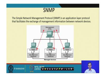
So, other another protocol which is there is a simple network management protocol SNMP is an application layer protocol, that facilitate exchange of management information between the 2 devices. So, SNMP is a application layer protocol, and it
