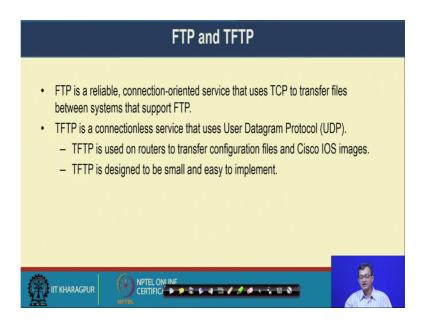
So, when we take the TCP FTP and TFTP. FTP is a reliable connection oriented service that uses TCP to transfer files between systems that support FTP, right. So, TCP FTP is a reliable connection oriented service right. Whereas, TFTP is a connectionless that uses UDP to transfer.
