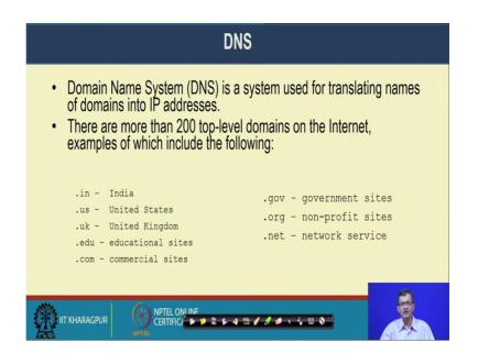
So, if we look at the DNS so, what is DNS? Domain Name Systems so, it is primarily major job is to translate name to IP like. So, when we because if you see the; if we I say that I want to find out www iitkgp ac dot in. Now www this name does not have any meaning at the IP layer or the down the layer right say whenever I want a routing the router requires a IP right. So, there should be there is either I give the IP at the top so that in understand this is the thing.
