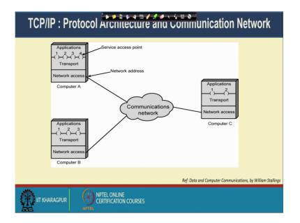
So, if we have a more holistic mix, where there are applications different applications. So, there are different service points of the things. So, this transport layer defines that, along with that we have a network access layer. So, IP plus the process allows me to run that application. So, that means, I may have a server which acts as a say FTP server, a SSI server or a Telnet server or different type of server. So, where the different things are define at different port.
