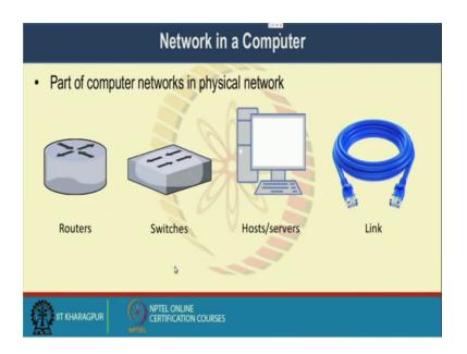
Now, here are the different parts or different components of computer networks in a physical network. So, you have the routers, you have the switches, you have different host and the server and you have the link.
