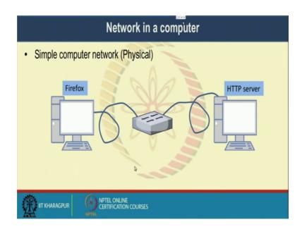
Now, this is a kind of simple computer network in the physical domain you have one host which is running say a browser like Firefox, it is connected to a network switch or a router that is again connected to a HTTP server. So, using the browser you can browse the data from the HTTP server.
