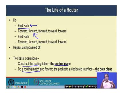
So, if you look into the lifecycle of a router apparently it is very simple. So, the lifecycle of a router is that you can represent it in the form of do repeat loop. So, you find a path to a particular destination, then you forward, forward, forward, forward, forward multiple packets to that destination again whenever a new destination comes you find out the path and then forward, forward, forward, forward the packets to that destination until the router gets powered off.
