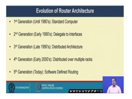
Well. So, this entire evolution of the router architecture, it came from 5 different generation starting from 1980s to today. So, the 5 generation of the router, so are just like a standard computer which we have a computer with multiple interfaces. The 2nd generation of the routers which came in early 1990s, they are delegate to interfaces. So that means, you have a router architecture where you will have multiple such interfaces at dedicated device.
