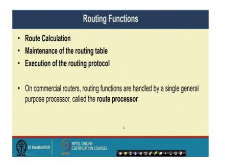
Now, the routing functions are basically there are 3 functionalities that you need to execute inside the control plane of a router, the route calculation based on a routing protocol, the maintenance of the routing table and the execution of the routing protocol. Now, in commercial routers, these routing functions are handled by a single general purpose processor which we call as the route processor that I have mentioned earlier.
