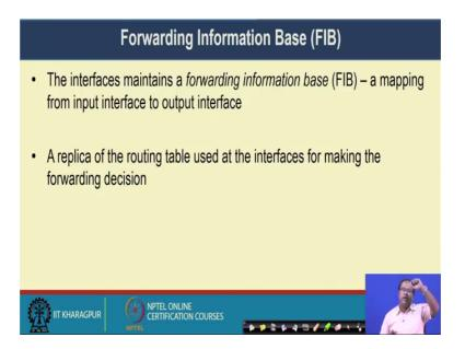
So, the interfaces they maintains a forwarding information base which is the local routing table. This forwarding information base is a mapping from the input interface to the output interface.
