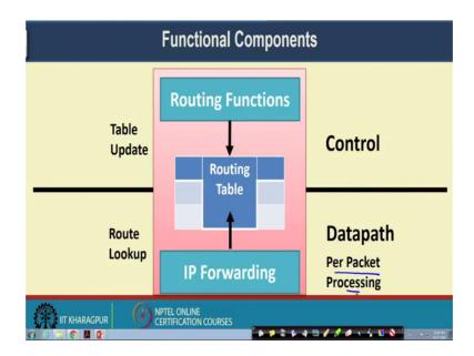
Now, let us look into the functional components of a router from the perspective of the control and the data path. You have the routing function and in the data path you have the IP forwarding as we have mentioned.
