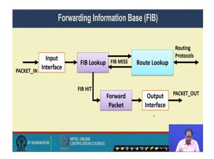
So, this is a the idea that whenever you have a packet in event; a packet in event means a packet is input to the system it is put into the input interface. In the input interface you look into the forwarding information base your local cache of the routing table which is implemented inside the hardware. After looking into this local cache, if there is a here; that means, the information is there in your FIB.
