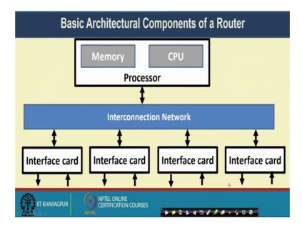
Well, so, this is the basic architectural components of a router. You have a processor, a general purpose processor which has a memory component and a CPU component. The processor is connected to multiple interface card. So, this network interface cards are the network interface card which are connected through a interconnection network inside your router hardware.
