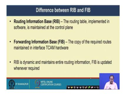
So, the difference between RIB and FIB is that the routing information base is the original software routing table which is a implemented in the software and maintained at the control plane. And forwarding information base is the copy of the required routes maintained at the interface of the TCAM hardware. Now, this RIB it is dynamic and maintains the entire routing information, whereas, FIB updated whenever required.
