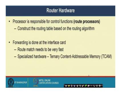
So, the router hardware the processor is responsible for the control function, we call it as a route processor. The control function means to run the routing program and then send the data packets over the network and construct the routing table.
