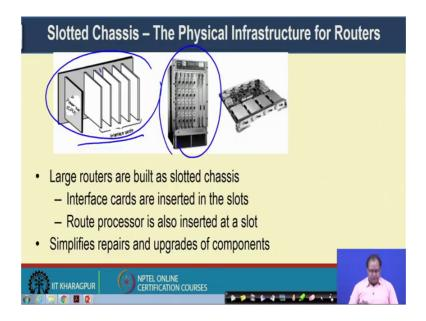
Now, if you look into the physical infrastructure of a router, we normally use something called a slotted chassis. So, this is a structure of a slotted chassis which are used to build up large routers. So, here is a structure of a chassis. So, you have this multiple chassis. So, individual interface card they are inserted inside these slots and then the route processor it is also inserted in a slot.
