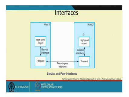
Now, so if you look at the very broad view interfaces. So, if you see there are some higher level objects right at the both ends. So, this is host 1, host 2; it can be directly connected or it can be at any level of the internet right. It can be machine to machines directly connected or two machines connected through different are different network and frame.
