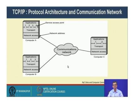
So, that single stack; that means, underlining physical layer physical communication path is there which takes care by these type of protocol. So, if we have a big picture. So, we have different computers where this applications through this transport service access point and there is network access. And we have a underling communication path which allows me to connect to this different devices across this internet.
