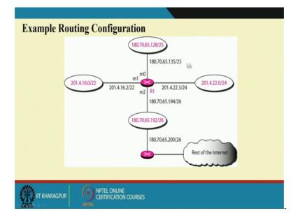
Like here what we are having, there are several network like starting point, 180 70 65 slash 25 here 20 14 dot 16 dot 0 and it is connected with different interfaces of this particular router right. So, it connected to the different phases of this router and there can be a default route, may one of this interface right.
