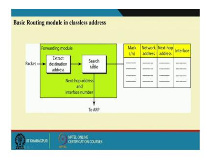
Now, if we look at the basic modules or very fundamental structure of the a particular router so, once it is received a packet you need to extract the destination address from the
