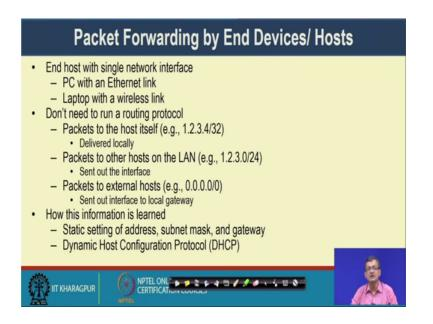
And packet forwarded by the forwarding packets, forwarded by there is a type of forwarded by the n devices or the host like. So, at what we are having at our end is the Ethernet link. This machine has some RJ 45 connection to the cable to the next things. So, PC with Ethernet links, laptops with wireless links, does not need to run a routing protocols. So, right it forward to that particular local or the next hop whatever the gateway is defined into the things right.
